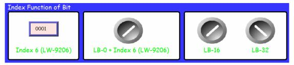
If Index 6 (LW-9206) is set to 1, then switch [LB-0 + Index6] reads LB-16 which is in ON state.
