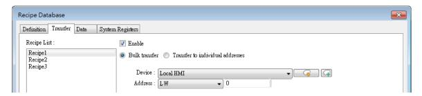
Under this mode, the data type settings of destination addresses must follow those of the recipe items. The following table shows the bulk transfer result when LW-0 is designated as the starting address given settings in the following figure.
