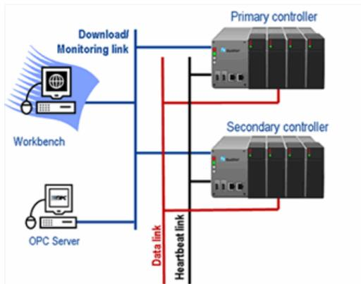
The failover mechanism consists of two devices (primary and secondary) executing the same application. At the end of each cycle, both devices synchronize their data by exchanging CRCs (data link). This parallel execution allows a bumpless switch-over between both devices. During execution, only one device is active. This device updates the output while the other device remains on standby. A heartbeat signal is sent between devices to ensure availability.
