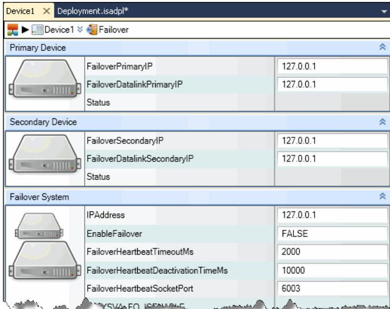
Configuring a failover mechanism consists of setting parameters defined by the OEM where some may differ depending on whether it uses an Ethernet, serial, or another link type. Since a failover mechanism requires Ethernet communication for the dialog between devices and the workbench, the configuration is similar for all implementations:
