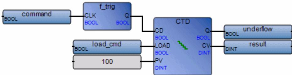
(\* ST Equivalence: We suppose F\_TRIG1 is an instance of F\_TRIG block and CTD1 is an instance of CTD block\*)
