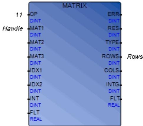
**Note:** The failover mechanism does not support the Matrix function blocks.
