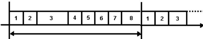
In a case where bindings are defined, variables consumed by a resource are updated after the inputs are scanned and the variables produced for other resources are sent before updating outputs.
