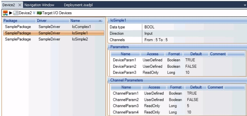
You can use direct variable representation (%IX1.1) to access I/O values when I/O channels have no wiring.
