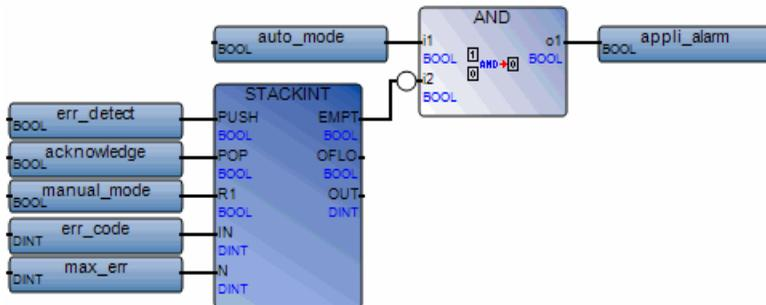
(\* ST Equivalence: We suppose STACKINT1 is an instance of STACKINT block \*)
