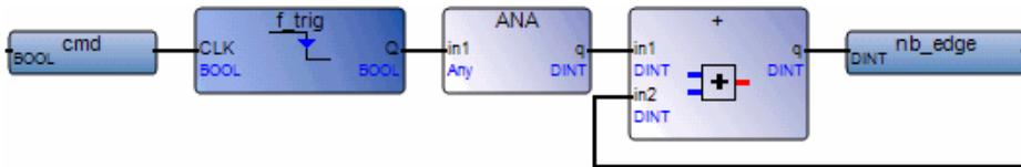
(\* ST Equivalence: We suppose F\_TRIG1 is an instance of F\_TRIG block \*)
