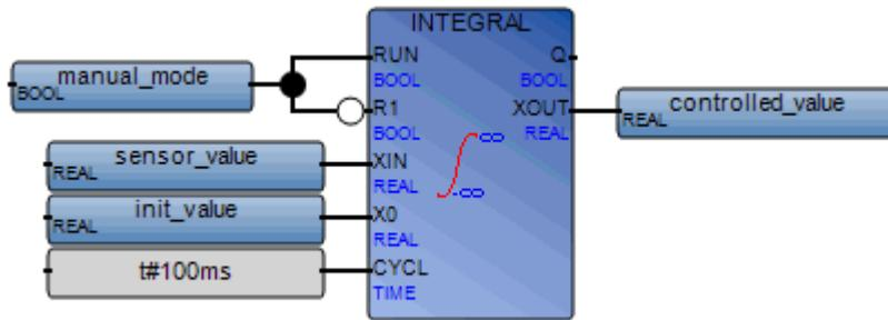
(\* ST Equivalence: INTEGRAL1 instance of INTEGRAL block \*)
