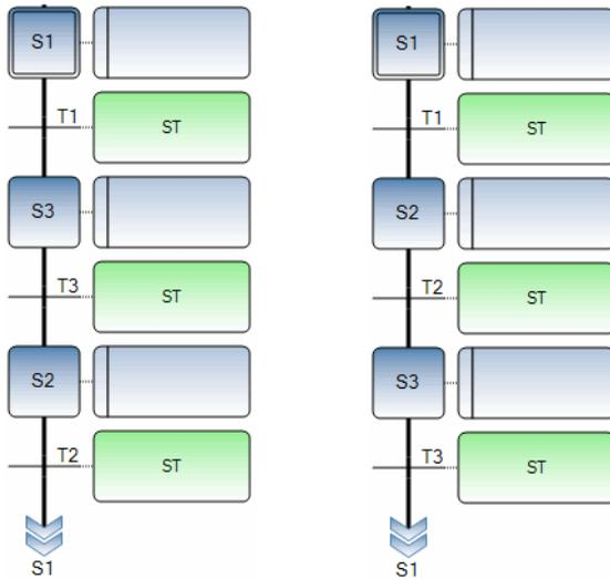
The following example shows the E\_Merge function block made up of an initial step, two transitions, and a step:
