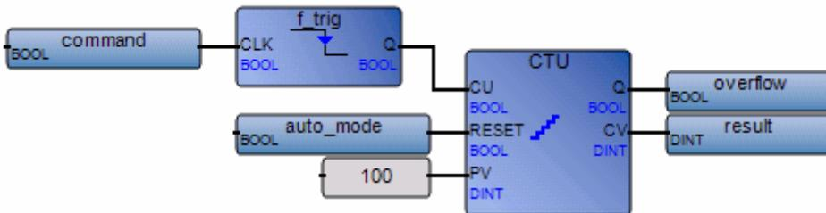
(\* ST Equivalence: We suppose R\_TRIG1 is an instance of R\_TRIG block and CTU1 is an instance of CTU block\*)
