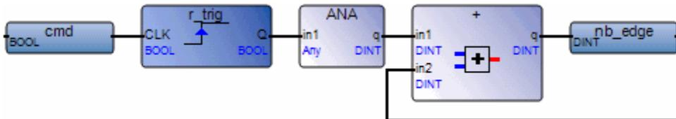
(\* ST Equivalence: We suppose R\_TRIG1 is an instance of the R\_TRIG block \*)
