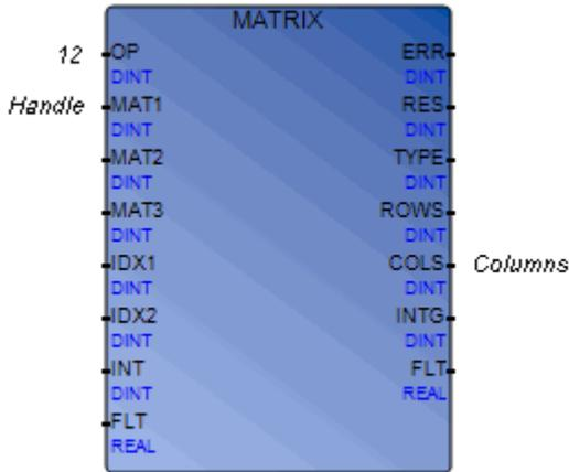
**Note:** The failover mechanism does not support the Matrix function blocks.
