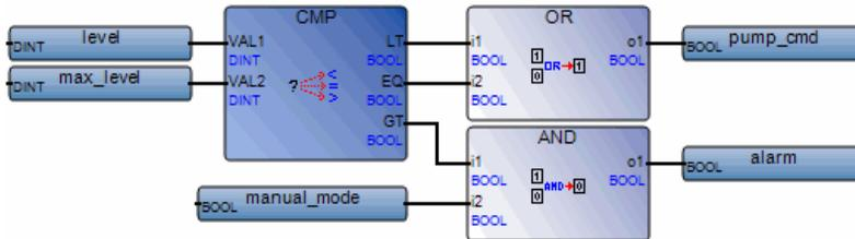
(\* ST Equivalence: We suppose CMP1 is an instance of CMP block \*)
