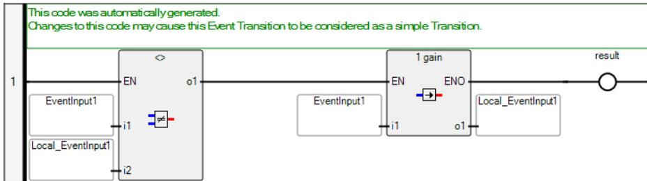
Transitions are represented by a small horizontal bar that crosses the connection link. Event transitions are displayed with an additional arrow pointing towards the connection link. Each transition is referenced by a name, displayed next to the transition symbol.
