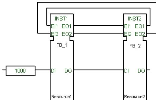
Insertion of an IEC 61499 basic function block or composite function block into a program is enabled following its creation in the project library.
