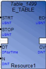
The parameters for standard IEC 61499 function blocks are displayed in the local variables instance with their equivalent direction attribute. The E\_TABLE function block shows the following directions for its inputs and outputs:
