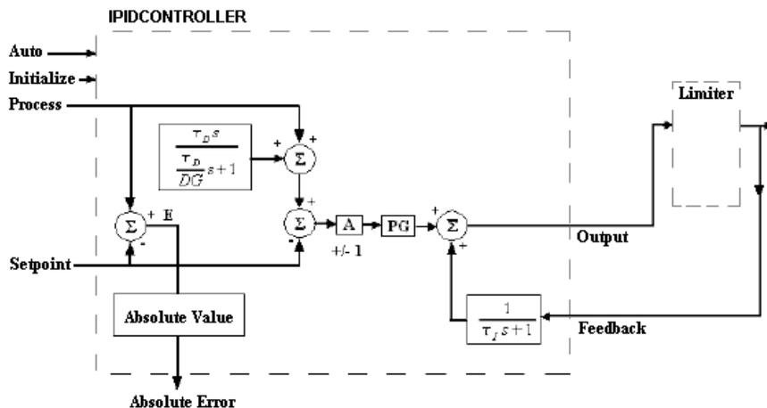
For Input Initialize, changing from Logic Zero (FALSE) to Logic One (TRUE) or Logic One (TRUE) to Logic Zero (FALSE) when AutoTune is Logic Zero (FALSE) causes the IPID element to eliminate any proportional gain action during that cycle (i.e Initialize). This can be used to prevent bumping the Output when changes are made to the SETPOINT using a switch function block.
