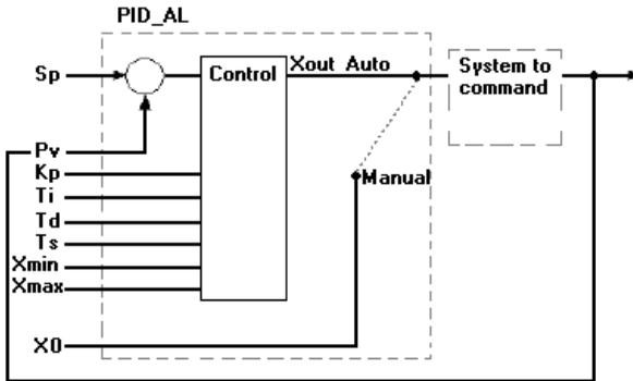
The PID\_AL function block is implemented using the following PID model:
