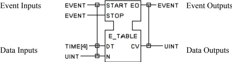
An IEC 61499 function block is represented by a box having an upper section representing the event control chart and a lower section representing the data process. Three names are indicated in the block: the instance name at the top, the function block name just below, and the resource in which it is declared at the bottom.
