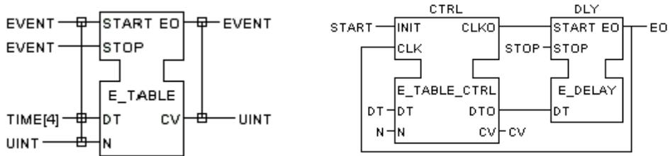
An event occurs at EO at an interval DT[0] after the occurrence of an event at EI. A second event occurs at an interval DT[1] after the first, etc., until N occurrences have been generated or an event occurs at the STOP input. The current event count is maintained at the CV output.
