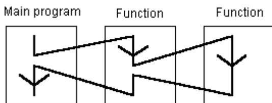
Any POU of any section can call one or more functions. A function can have local variables.
