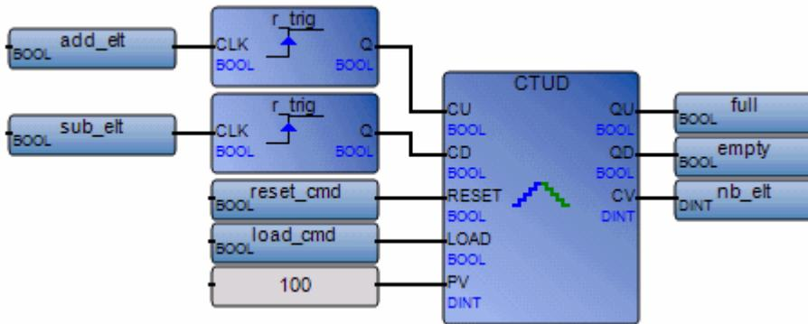
(\* ST Equivalence: We suppose R\_TRIG1 and R\_TRIG2 are two instances of R\_TRIG block and CTUD1 is an instance of CTUD block\*)
