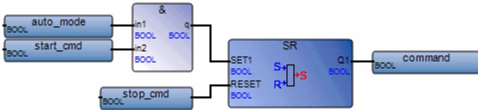
(\* ST Equivalence: We suppose SR1 is an instance of SR block \*)
