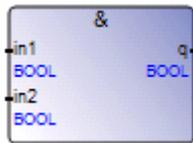
**Note:** For this Operator, the number of inputs can be extended to more than two.
