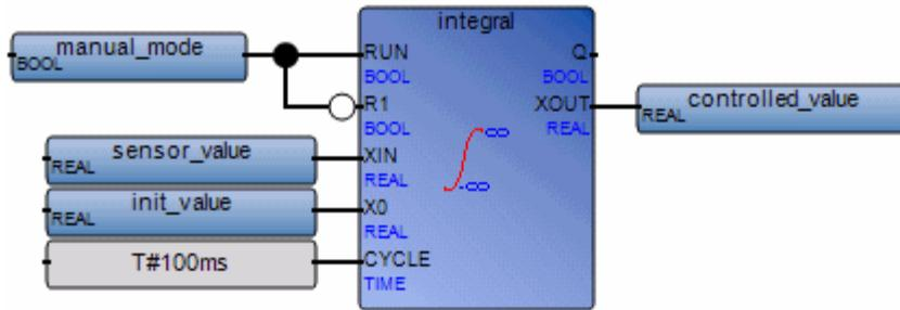
(\* ST Equivalence: INTEGRAL1 instance of INTEGRAL block \*)
