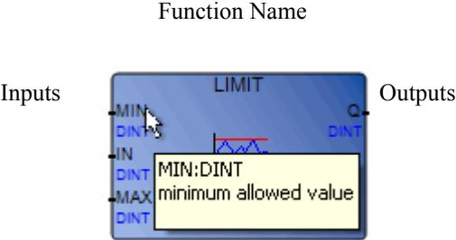
Input variables of an FBD program must be connected to input connection points of blocks. The type of each variable must be the same as the type expected for the associated input. An input for FBD diagram can be a literal, any internal or input variable, an output variable, or a block output.
