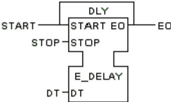
An event occurs at EO at an interval DT after the occurrence of an event at START, and at intervals of DT thereafter until the occurrence of an event at STOP.
