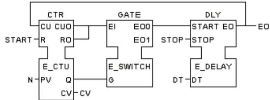
An event occurs at EO at an interval DT after the occurrence of an event at EI, and at intervals of DT thereafter, until N occurrences have been generated or an event occurs at the STOP input.
