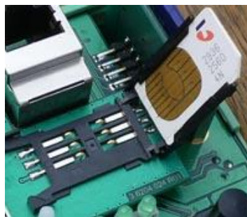
Figure 2.7: SIM card placement in an M3G.
