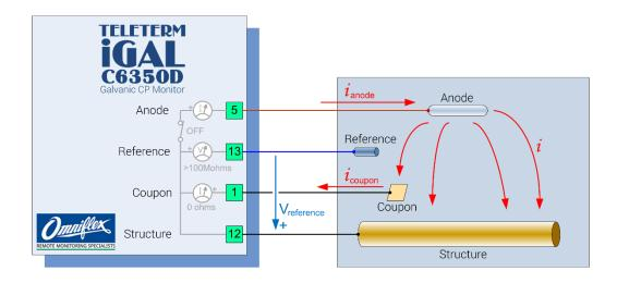
This diagram shows the flow of currents and presence of voltages when the iGAL is installed in a galvanic CP system. (Note the direction of flow of current out of the anode and into the coupon)
